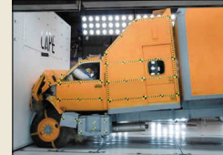
Barrier crash test
